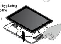
**8** While pressing the latches on the stand, slide the sleeve into the stand.
